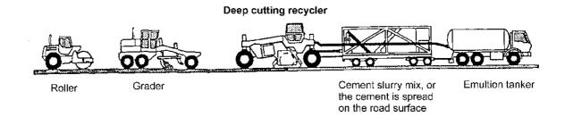
The configuration of the recycling train where cement is used together with bitumen emulsion is shown in the diagram above.
