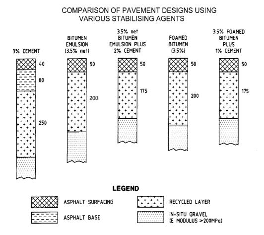
The choice of stabilising agent has a significant impact on the pavement cost, as the stabilising agent itself is normally the largest component in the total recycling cost. In order to evaluate the most cost-effective design for a particular project it is therefore necessary to carry out pavement designs using each of the stabilising agents. Cost comparisons can then be made based on the thickness of the layers required using local rates for the various stabilising agents.
