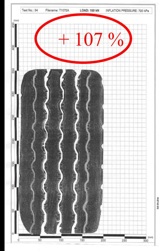
**Figure 6: Static Tyre Foot Prints**
