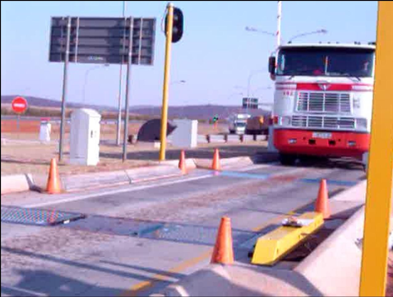
In operation: Quad (full) SIM pad configuration at a typical weighbridge site on National Road 3 (N3), near Heidelberg in Gauteng.
