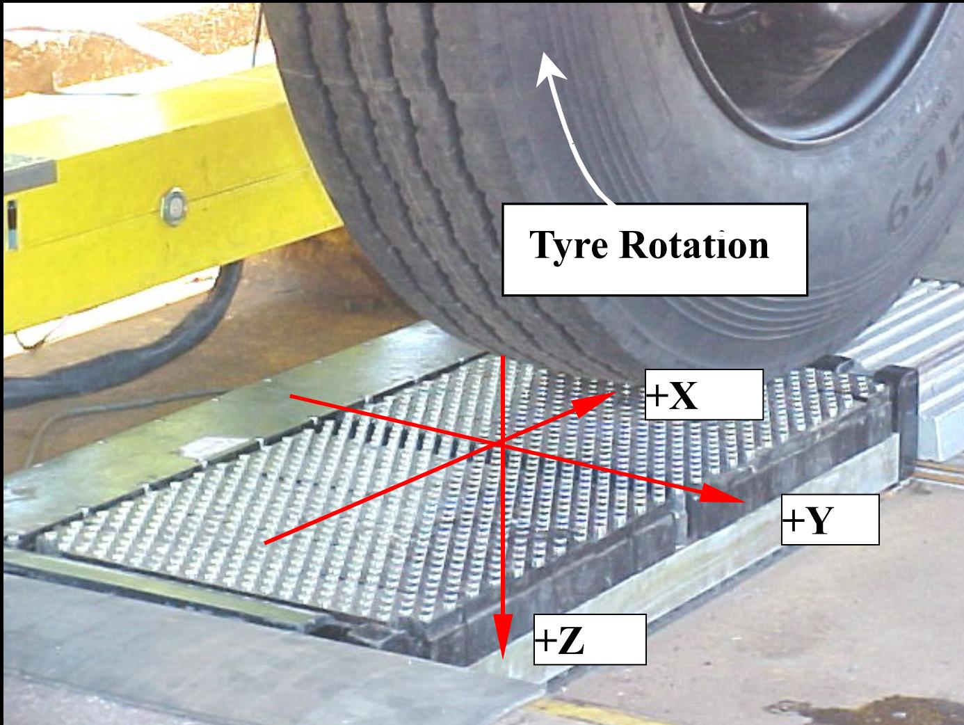
Figure 4: SAE sign convention used during SIM measurements.
