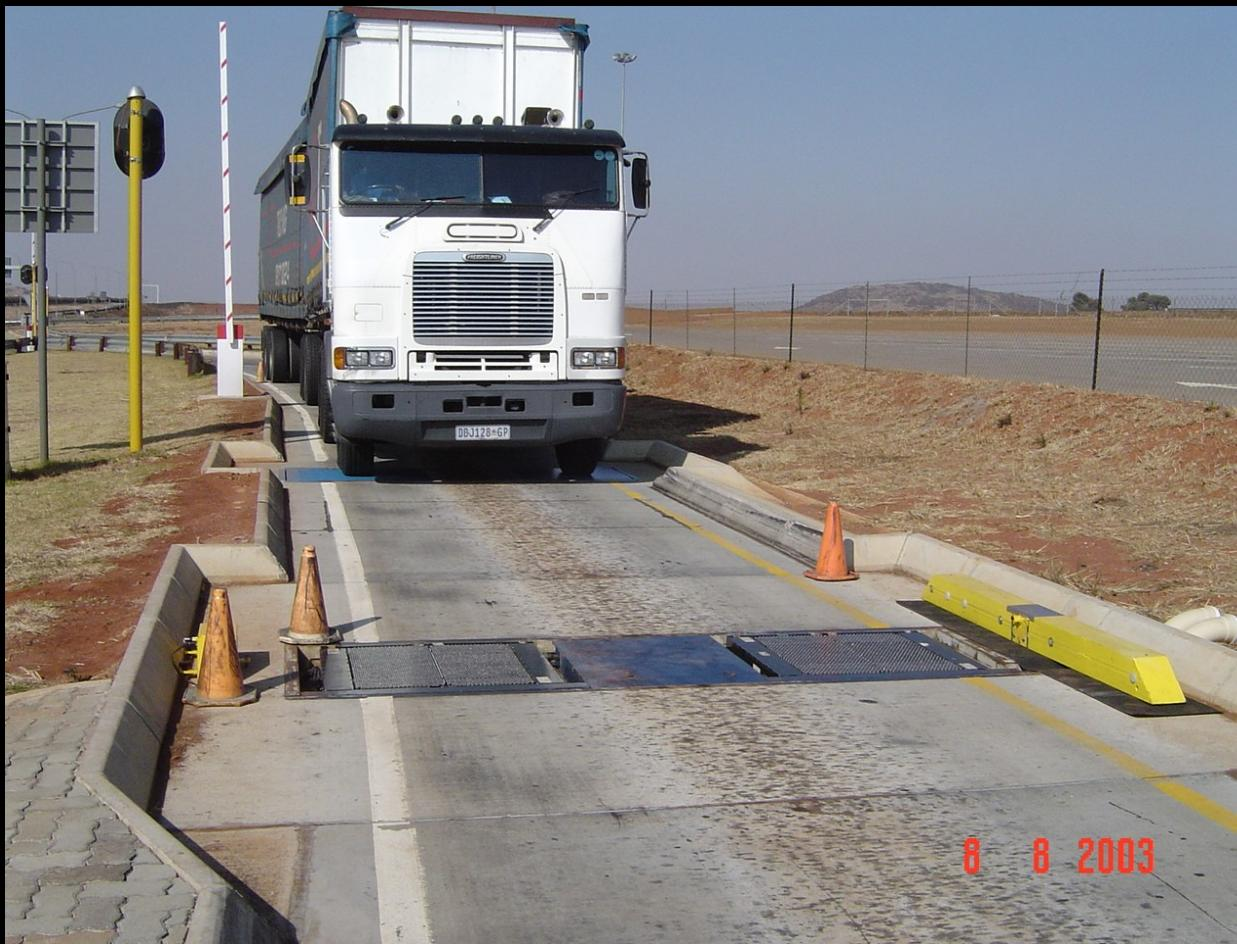
Figure 2: Quad (full) SIM pad configuration at a typical weighbridge site on National Road 3 (N3), near Heidelberg in Gauteng.
