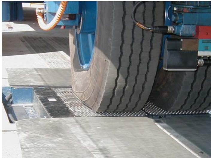
Figure 6. Twin (or dual) SIM pad configuration (used under Heavy Vehicle Simulator (HVS) with dual test tyres).
