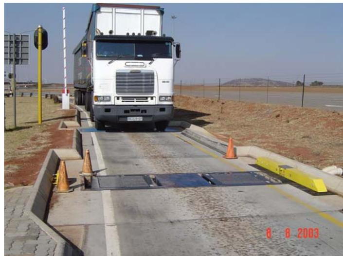
Figure 7. Quad (full) SIM pad configuration at a typical weighbridge site on National Road 3 (N3), near Heidelberg in Gauteng.
