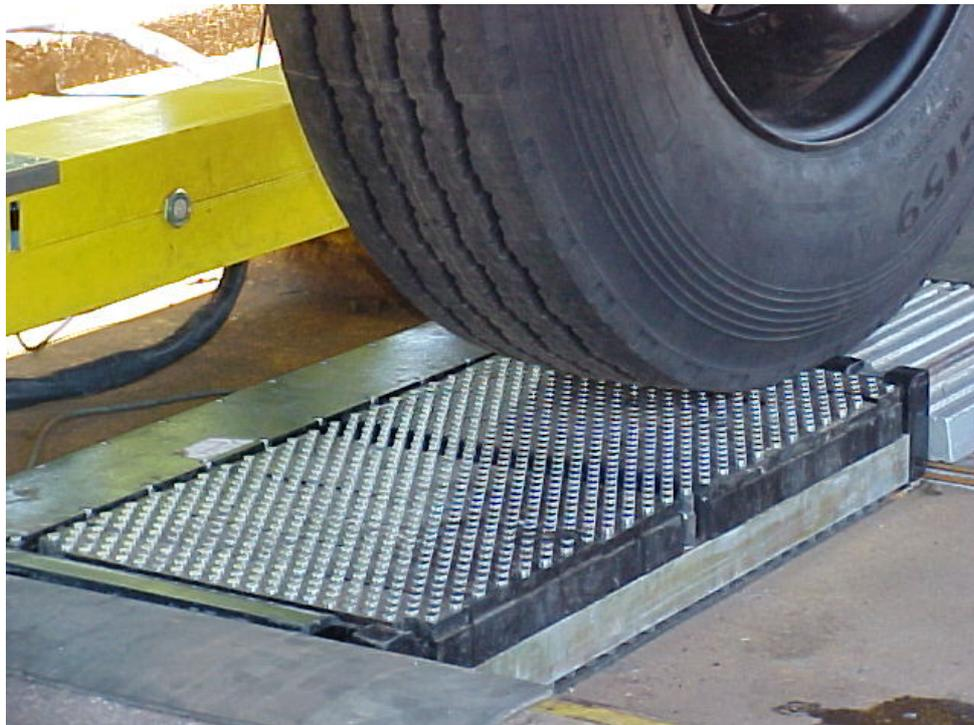
**Figure 5. Single SIM pad configuration (used under Heavy Vehicle Simulator (HVS) with single test tyre).**
