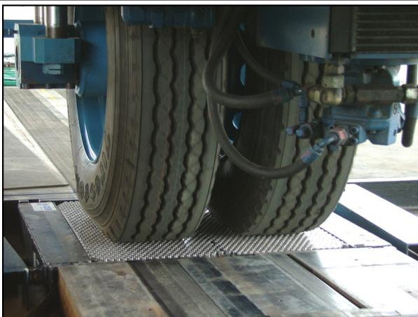
**Figure 3. HVS full-scaled dual tyres on the rough-textured SIM surface.**
