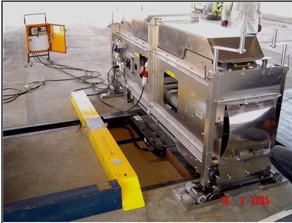
**Figure 1. MMLS3 on the SIM pad at GDPTRW, Koedoespoort facility.**
