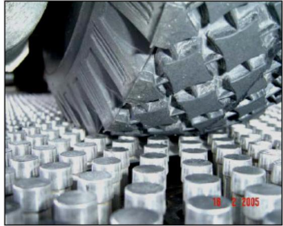
**Figure 2. Close-up: 1/3<sup>rd</sup> scale D-tyre of MMLS3 on the rough-textured SIM surface (pad).**
