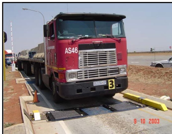
Figure 1 – Typical heavy vehicle (HV Class 1:2:2:2) moving slowly over the SIM device during measurement. Note the two SIM pads each side in front of the tyres.
