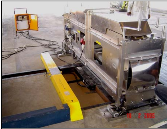
Figure 3. MMLS3 on the SIM pad at GDPTRW, Koedoespoort facility.
