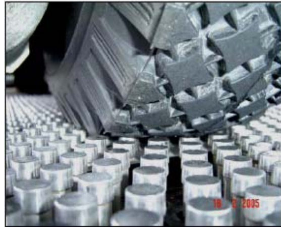
Figure 4. Close-up: 1/3 rd scale D-tyre of MMLS3 on the rough-textured SIM surface (pad).
