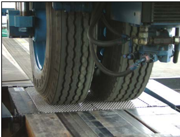
Figure 5. HVS full-scaled dual tyres on the rough-textured SIM surface.
