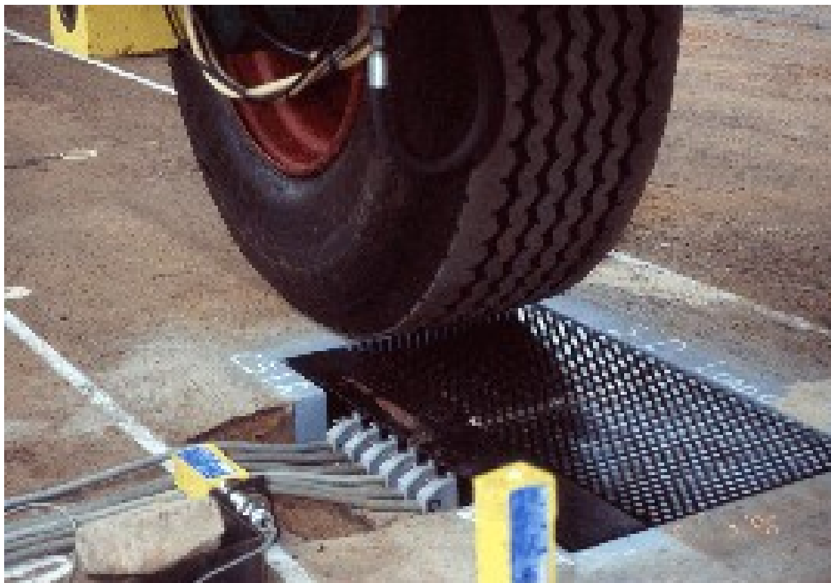
315/80 HVS TYRE ON SIM Mk II SYSTEM
